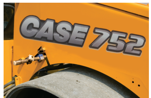
New sprinkler nozzles with built-in filter
