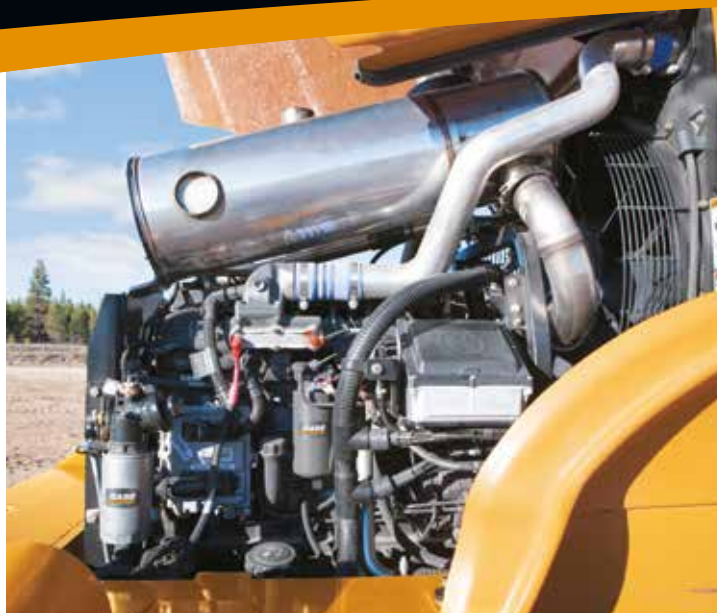
The layout of the components under the hood is optimized and results in easier maintenance.
